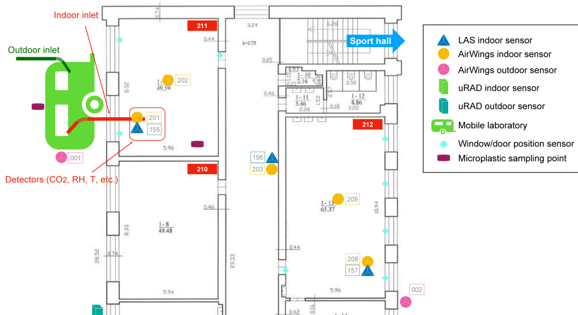
Figure 6 Location of LCS devices and state-of-the-art instrumentation in the school site of Vilnius campaign.
