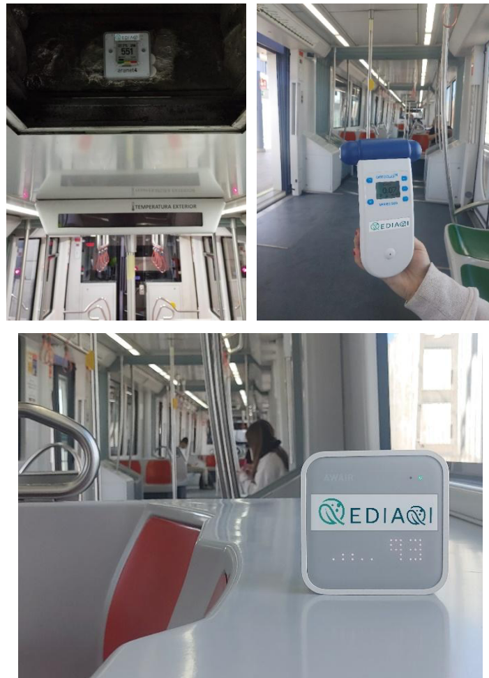
Figure 28 Measuring devices used inside the metro train.
