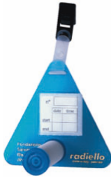
Figure 2 Radiello passive sampler (left) and NetPID station (right)
