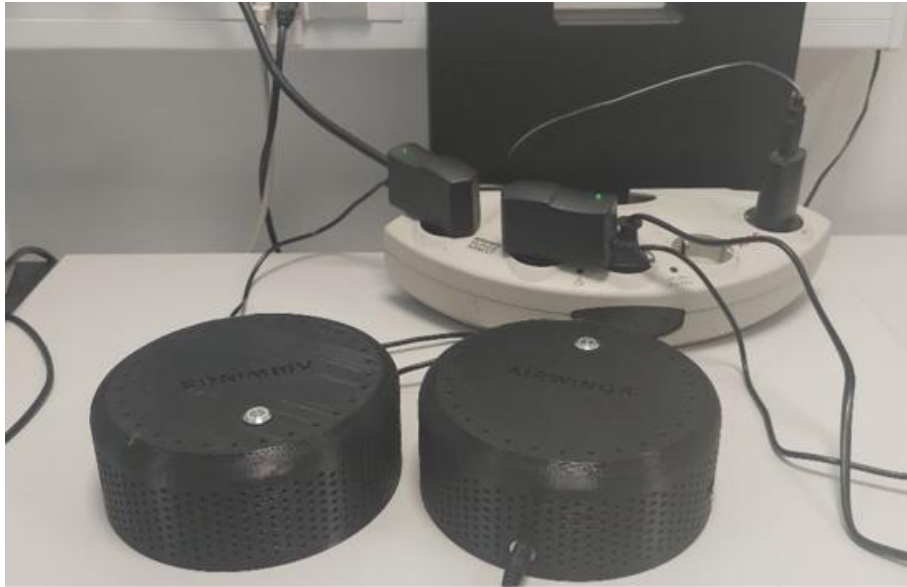
Figure 11 - AIRWINGS Environmental Monitoring System
